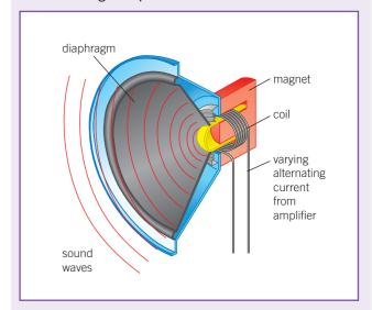
A coil of wire is placed inside a permanent magnet (so it is inside a magnetic field) and is attached to a diaphragm.
