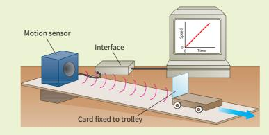
As the trolley accelerates down the runway, the velocity increases with time. Therefore, the line on the graph will go up and remain straight to suggest that the acceleration of the trolley is constant.
