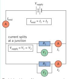
The total resistance of two or more components in parallel is always less than the smallest resistance of any branch. This is because adding a loop to the circuit provides another route for the current to flow, so more current can flow in total even though the p.d. has not changed. Adding more resistors in parallel decreases the total resistance of a circuit.
