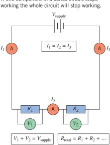
Components with a higher resistance will transfer a larger share of the total p.d. because V = IR (and current is the same through all components).
